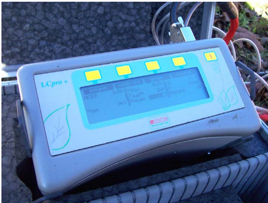
Figure 1c. Display unit showing NCER value and soil temperature (Tsoil m).
